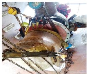
After jobs were completed at the workshop, it was brought and installed on the vessel, propeller blades connected, all systems tested, thruster grid installed, and in a very efficient manner, vessel was ready to depart.
