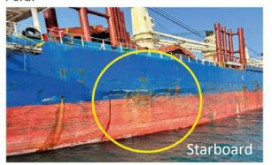
A vessel hit her causing ruptures and major deformations on the port and starboard sides in the way of the stern area below the superstructure of the vessel. We were immediately contacted by the owner's superintendent who immediately got on a plane to visit the vessel and requested us to perform an on-site assessment of damages.
