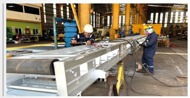
Talleres Industriales has been certified and holds the needed expertise to carry out repairs on gangways and accommodation ladders. We have class-approved certifications and procedures to perform aluminum structural welding repairs as well as the replacement of damaged profiles.
