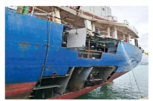
Also, a complete deck on the superstructure which included davits, a winch, ventilation system, and piping were renewed.
